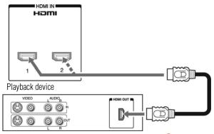
(Sample Illustration) Connecting an HDMI® device
