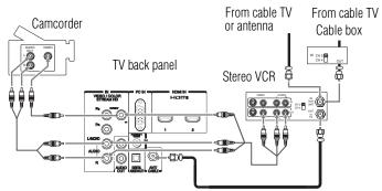
(Sample Illustration) Connecting to a VCR, antenna, cable TV, or camcorder
